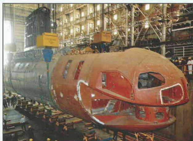
Lifting and shifting of Section 4 of Submarine-1 on Pontoon.
